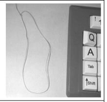
Slip the loop under and at the <u>center</u> of the keycap, and pull <u>straight up</u> with a quick, strong snap. Repeat for the remaining 25 alpha
